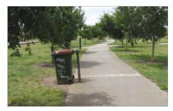
Figure 4: Rubbish bin and post causing a hazard for cyclists
