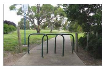
Figure 3: End of path treatments can present a hazard to cyclists
