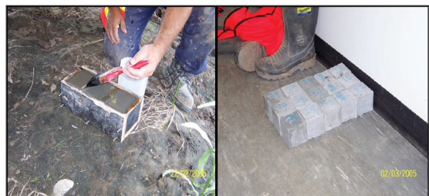
Fig 3: Making of cementitious mortar and grout test cube samples with exposed surface cured with the application of a curing compound (L), Test cube samples awaiting transportation to the laboratory for curing under laboratory-controlled conditions and subsequent testing for compressive strength (R)
