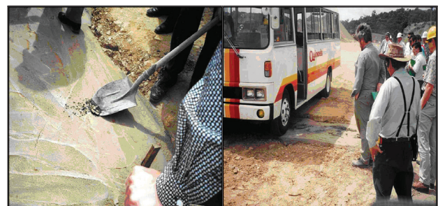
Fig. 3 Low strength flowable fill can be re-excavated using hand tools (L), Higher strength flowable fill loaded by small bus wheels
