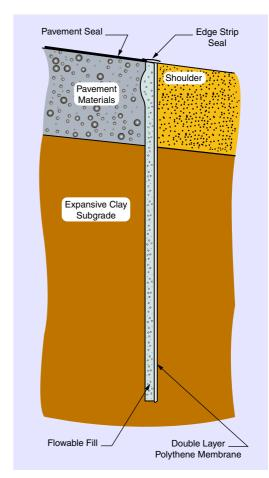
Figure 1. Cross-section of Barrier
