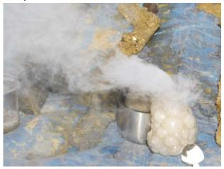
Figure 6: Using hot water to accelerate oxidisation of soil with hydrogen peroxide solution.
