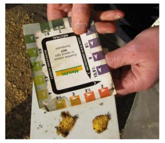
Figure 5: Measuring pH of insitu soil samples.
