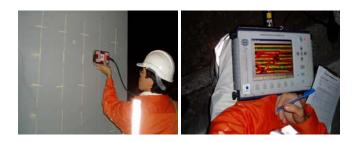
*Figure 1 - Ground Penetrating Radar (GPR) testing utilising high frequency impulse radar*
