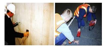
Figure 2- Cover meter measurements, concrete column (Left) and concrete deck overlaid with asphalt (Right)
