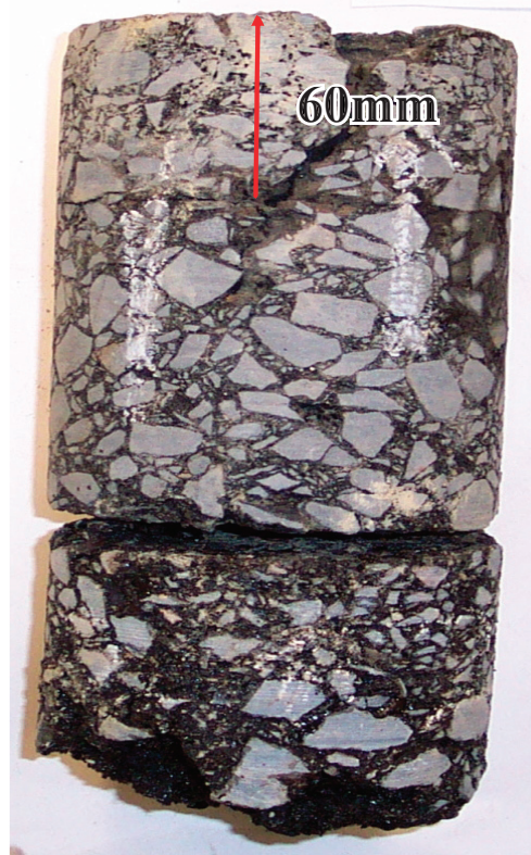
Figure 1 Example of extent of cracking and condition of underlying asphalt.
