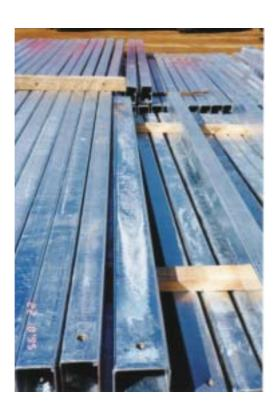
Figure 8.1: The storage of galvanized components should allow for air circulation, to avoid wet storage stain and formation of white zinc corrosion product.
