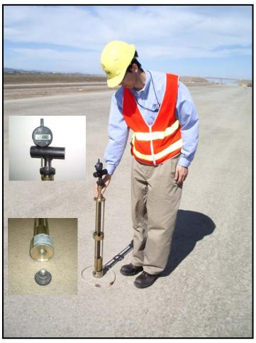
Figure 10 : Ball Embedment Penetrometer
