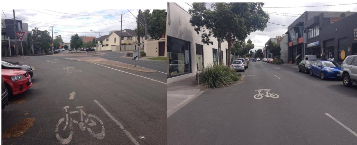
The above photo shows 'sharrows' being used to transition from a dedicated on-road bicycle facility into a low speed roundabout.
