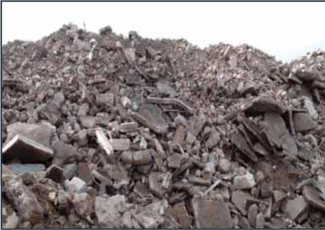
Figure 2: Reclaimed concrete for crushing, screening and removal of contaminants
