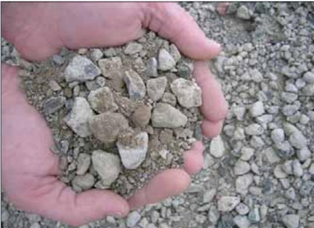
Figure 3: Crushed concrete
