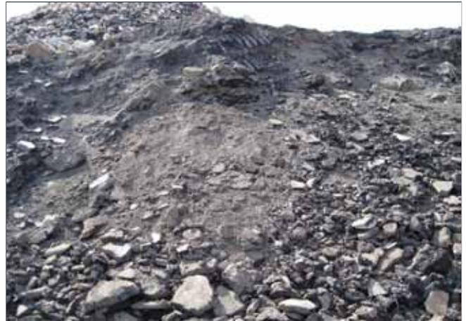
Figure 4: Reclaimed asphalt for crushing
